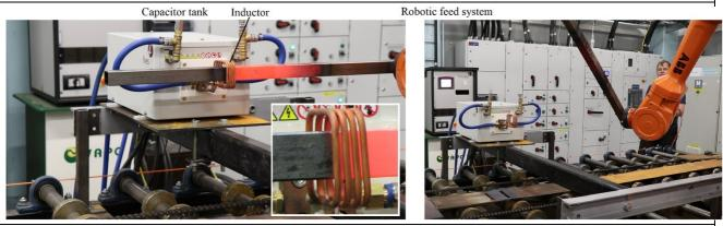
Fig. 7. The updated MP25 unit (capacitor tank + inductors) showing a coil for rectangular pipes as an example.
