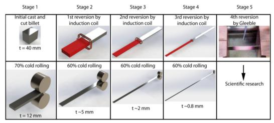
Fig. 54. Schematic illustration of experimental setup for multiple reversion treatments.
