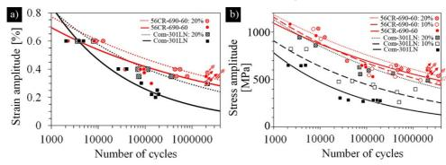
Fig. 41. Total strain amplitude vs number of cycles to failure (a) and mid-life stress amplitude vs. number of cycles to failure (b). The runover (2e6 cycles cut-off) specimens are shown in the inserts with the different y-axis scale. Load in RD direction. Coding e.g.: 56CR, 56% prior cold rolling reduction; -690, 690°C maximum temperature; -60, 60 seconds until self-cooled to 600 °C; :20%, 20% cold rolling. [Antti Järvenpää, PhD thesis 2019]
