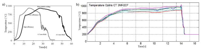
Fig. 23. Temperature measurement results from induction hardening experiments showing a) MP600 performance with 4.2 (1.3 m/min) and 6.5 mm (0.75 m/min) thick B27 boron steel (thermocouples) and b) "Laboratory unit" performance with 2.0 mm thick B24CR steel (pyrometer).
