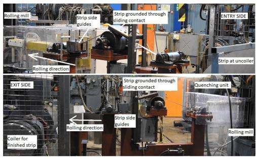
Fig. 16. The actual experimental setup in the MEFOS facilities.
