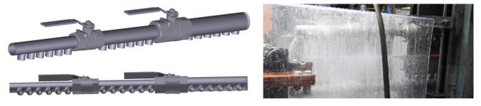
Fig. 18. Quenching unit designed and manufactured by the community for the simulation of DQ and DQ&P.
