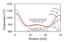
Fig. 24. Temperature distribution in continuous annealing without hot rolling using 2 mm thick B24CR steel with Coil Design v.2. The average temperature in the center is approximately 890 °C.
