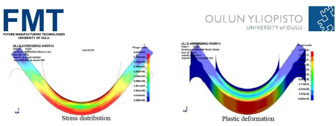
Fig. 52. Stress and strain distribution in bending process. Test material yield strength 960 MPa. [Antti Järvenpää, Master's thesis]
