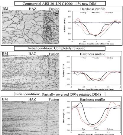
Fig. 43. The microstructure and hardness profiles for welded AISI 301LN.
