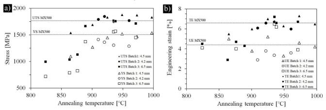
Fig. 26. a) Tensile strength and b) elongation for induction hardened B27 steel after annealing (MP600) at various maximum temperatures followed by water quenching. MX500 = commercial Miilux 500 steel grade. Sample size in annealing experiments 4.2–6.5 x 400 x 1000–2500 mm (t x W x L) and in tensile tests 12.5 x 50 mm (W x L, gauge section).
