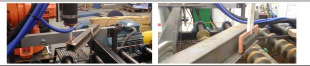
Fig. 9. The updated MP25 unit (capacitor tank + inductors) showing a coil for annealing outer corners (welded structures) as an example.
