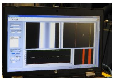
Fig. 21. Graphical user interface - measurement of strip position /control strip steering /mill tilt.
