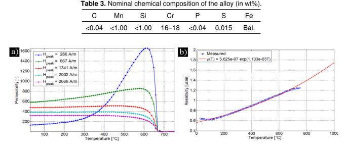
Fig. 36. (a) Measured temperature dependency of the permeability at peak magnetic flux density and (b) measured resistivity (blue circles) and parametrized temperature dependency of the resistivity (red line).
