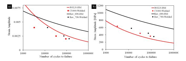
**Fig.44.** Fatigue life for annealed and welded AISI 301LN structures. The monotonic yield strength of the welded structures is the same (629 MPa). Data for annealed reference structures commercial 301LN and 56CR-690-60 are taken from Section 1.3.2 (Fig. 41).
