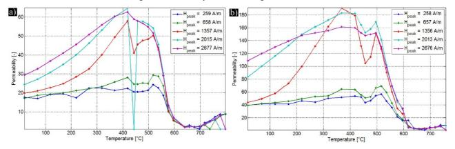
Fig. 46. Measured temperature dependency of the permeability at peak magnetic flux density for a) 32% and b) 56% cold rolled AISI 301LN.
