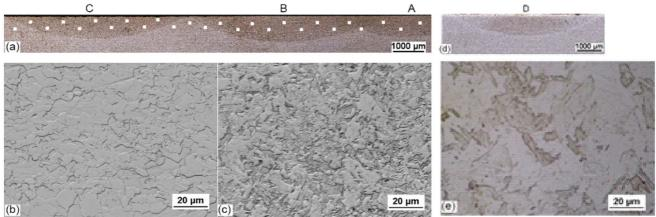
**Fig. 48.** a) Macrostructure of hardened tracks. b) Microstructure of base material which is completely ferritic. c) Microstructure of hardened track which is martensitic d) Single track with higher power input and e) more coarse martensite structure formed by the higher power.
