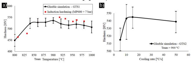
Fig. 27. Average hardness of the Gleeble hardened B27 steel showing the effect of a) annealing temperature (red squares showing induction hardened counterparts) and b) cooling rate. Sample size in annealing experiments 4.5 x 10 x 50 mm (t x W x L).
