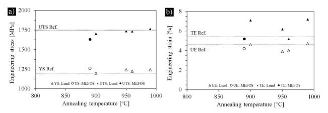
Fig. 28. a) Tensile strength and b) elongation for induction hardened B24CR (2 mm) steel after annealing (MP600) at various maximum temperatures followed by water quenching. Ref. water quenched (from 925 °C) B24CR. Sample size in annealing experiments in Lund 2 x 114 x 500 mm (t x W x L), in MEFOS 2 x 30 x 5000 mm (t x W x L) and in tensile tests 12.5 x 50 mm (W x L, gauge length).
