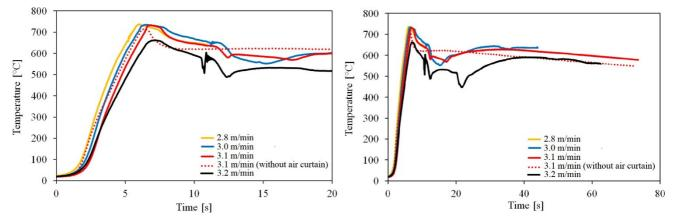
Fig. 29. Temperature measurement results for induction tempering tests in Nivala (MP600). Sample size in annealing experiments 8 x 400 x 1500 mm (t x W x L).
