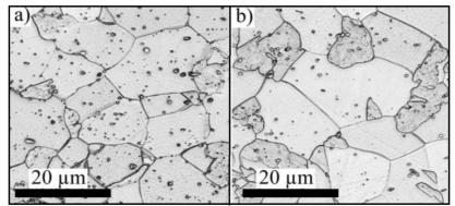
Fig. 35. Grain structure of a specimen heated at 500 °C/s and annealed for 10 s at (a) 925 °C and (b) 950 °C showing ferrite and martensite (darker grains) and chromium carbides.
