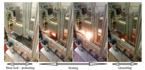
Fig. 11. "The laboratory unit" at the Lund University. Transverse inductor with sheet transfer system and quenching tank.
