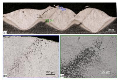
Fig. 51. (a) Macro-image of deposited tracks. (b) Area close to the surface. (c) Area where the melt transitions into base material.
