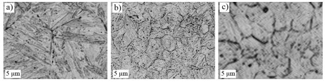
Fig. 25. Prior austenite grain structure for a) commercially hardened B27, b) induction hardened B27 (MP600) and c) Gleeble hardened B27.
