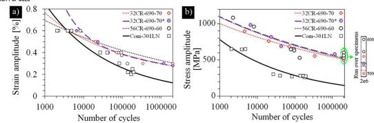
Fig. 40. Total strain amplitude vs number of cycles to failure (a) and mid-life stress amplitude vs. number of cycles to failure (b). The runover (2e6 cycles cut-off) specimens are shown in the inserts with the different y-axis scale. Load in RD direction. Coding e.g.: 32CR, 32% prior cold rolling reduction; -690, 690°C maximum temperature; -70, 70 seconds until self-cooled to 600 °C. [Antti Järvenpää, PhD thesis 2019]
