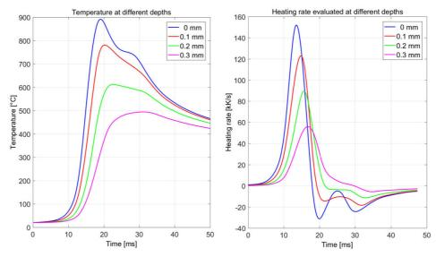
Fig. 53. Simulation results of the temperature (left) and heating/cooling rates (right) at four different distances from the surface for different time steps or positions of the strip during a transient heating operation with useful power of 30 kW and a strip speed of 1 m/s.
