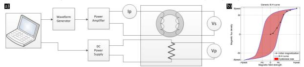
Fig. 13. a) Schematic illustration of the measurement setup. Ip is the excitation current, Vs is the induced voltage. 4-wire resistance measurement is supplied by a constant DC current and Vρ is the sensed voltage drop. b) Generic B-H curve illustration with remanence, coercivity and hysteresis loss as well as the initial magnetization curve.
