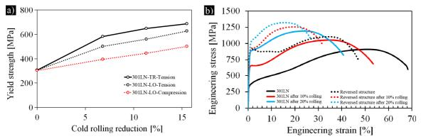
Fig. 38. Monotonic properties for cold rolled and reversed AISI 301LN showing a) anisotropy in cold rolled conditions and b) tensile test curves.
