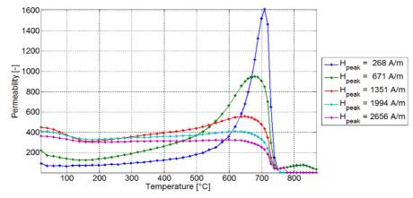
Fig. 33. Measured temperature dependency of the permeability at peak magnetic flux density.
