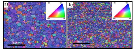
Fig. 34. Cross-sectional microstructure of a specimen heated to 950 °C at 25 °C/s for 10 s (a) and 500 °C/s (b) showing clearly finer fully recrystallized grain structure in rapidly annealed structure.
