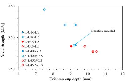
Fig. 36. The Erichsen index in relation to yield strength for AISI 430 and 441 steels both in commercial and laboratory annealed conditions (coded F-xxx). Punch speeds of 0.5 mm/s (LS) and 100 mm/s (HS) were used. Sample size 50x200 mm
