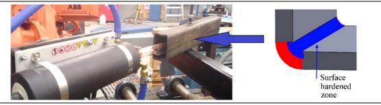
Fig. 8. The updated MP25 unit (capacitor tank + inductors) showing a coil for annealing inner corners (formed structures) as an example.
