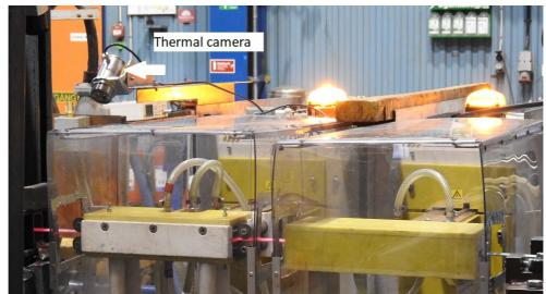
Fig. 17. Quenching unit designed and manufactured by the community for direct quenching (DQ) and direct quenching and partitioning (DQ&P) processes.
