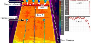
Fig. 30. Thermal imaging during induction tempering of 8 mm 1100 DQ&T. The line was running in reversed direction to allow the use of thermal camera and also to prevent air curtain to cool the surface of the sheet.
