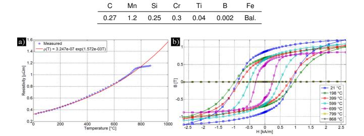
Fig. 32. (a) Measured resistivity (blue circles) and parametrized temperature dependency of the resistivity (red line) and (b) full hysteresis loops with Hpeak = 2656 A/m.
