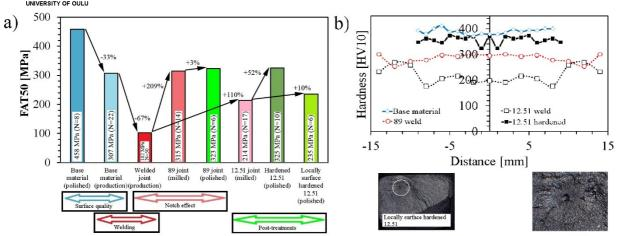
Fig. 47. Fatigue limit (FAT50) determined from S-N curves and b) hardness along the weld cross-section (top layer). The microstructural inserts show a subsurface crack initiation in surface hardened 12.51 joint after approximately 100 000 cycles. Esab OK Autorod 12.51 and Esab OK AristoRod 89 wires with 1.2 mm diameter.
